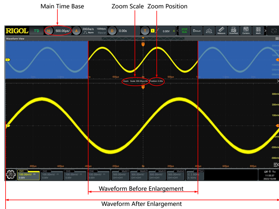
Figure 6.2 Delayed Sweep Mode
