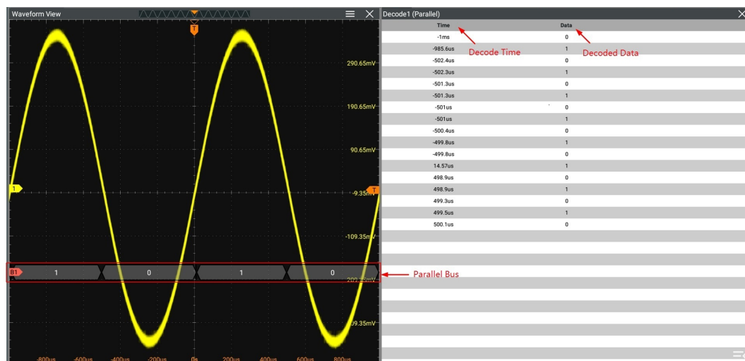
Figure 17.3 Parallel Decoding Event Table
