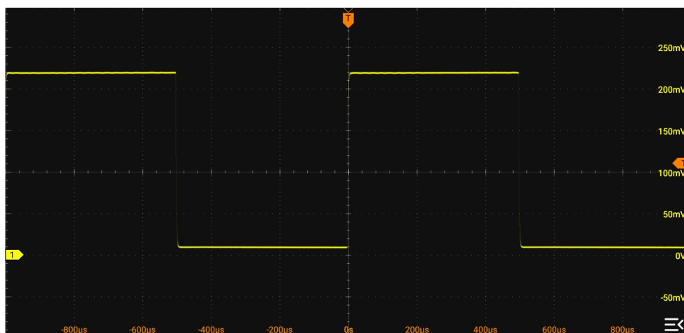
Figure 4.8 Square Waveform Signal
