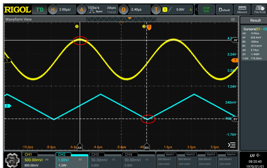
Figure 10.13 Track Measurement (after Horizontal Expansion)
